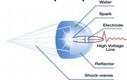
Acoustic waves are generated by an underwater high-voltage spark, which creates single pulse waves with high-pressure amplitude, small pulse width, and short rise time.
