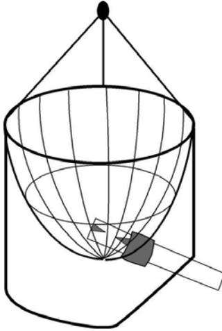
The electrohydraulic method uses a high voltage spark gap. The spark generates a plasma bubble that compresses the liquid, initiating the pressure wave. Each mechanism creates a characteristic waveform and energy density.
