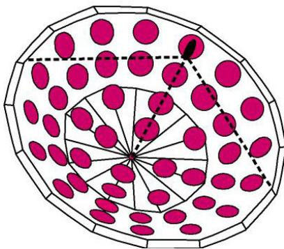
The piezoelectric system utilizes a crystalline material, that when stimulated with high voltage electricity can expand or contract to initiate a pressure wave in the surrounding fluid. The crystals are arranged so that the pressure wave is aimed towards a focal point.
