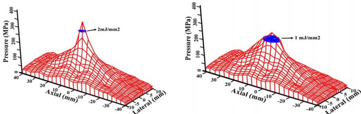
The figure on the left shows a high energy density associated with a fine focal point. On the right the same total energy is distributed to a large focal point resulting in a lower energy density.
