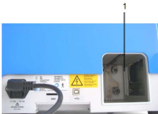
Figure 17 Pit for water cartridge (1)
