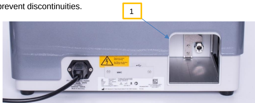
Figure 17 Pit for Water Cartridge (1).
