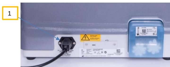
Figure 12 Installation of Power Supply.
