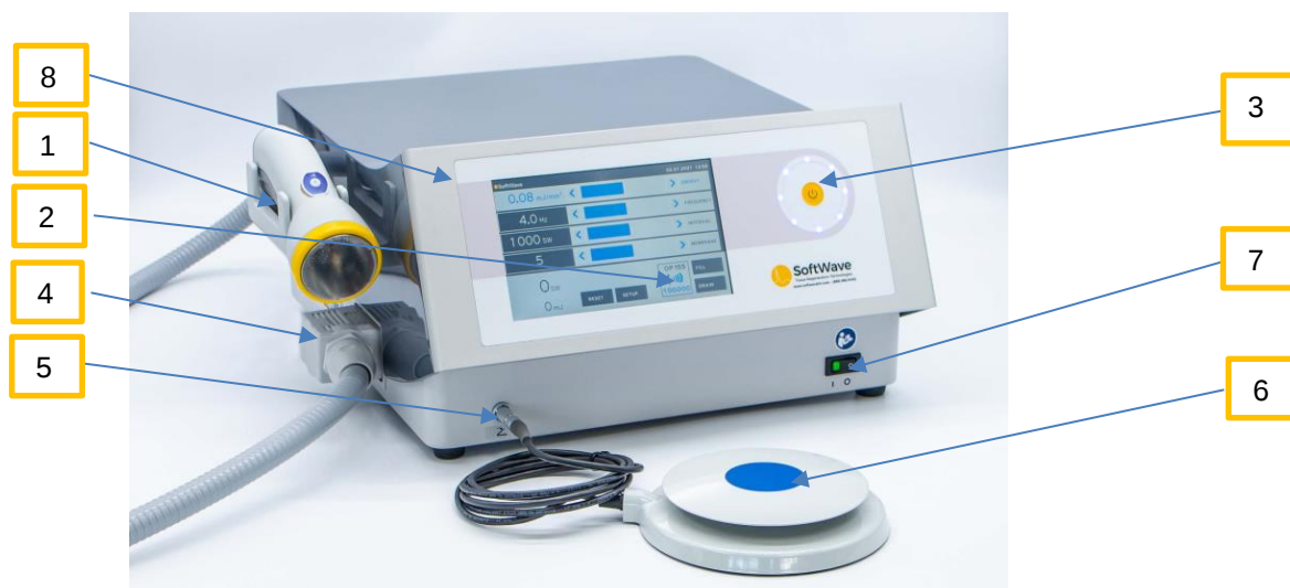
Figure 2 Components and Connections of the OW100-US at the Front Side.
