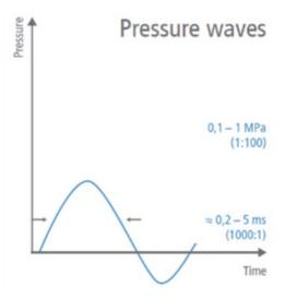
Radial pressure waves are acoustic pneumatic pulses with a low steeping effect, slow rise time with comparatively large negative pressure (tensile wave).
