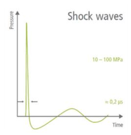
Shockwaves are acoustic pulses with high positive pressure, **fast and steep rise time** followed by comparatively **small negative pressure** (tensile wave).
